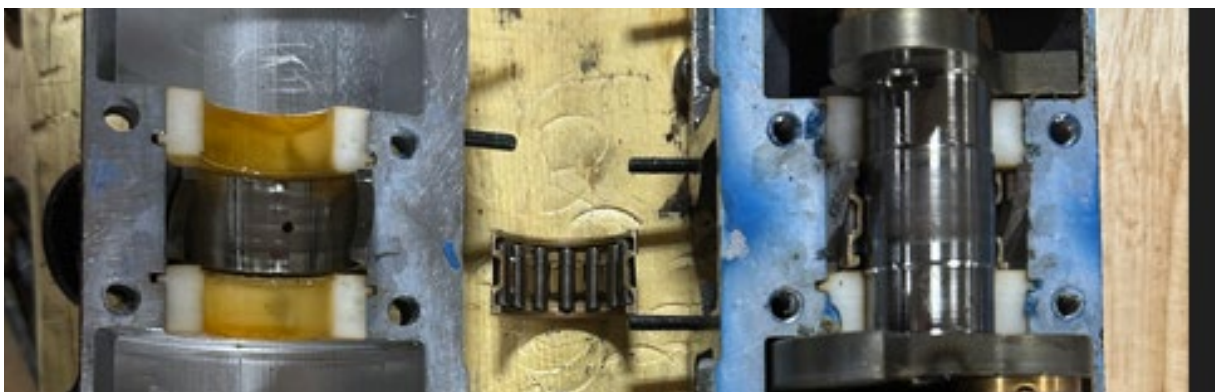
Figure 12. Main bearing wear.
