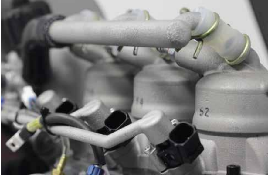
Three injectors spray heavy fuel at 3 bar into each of the three sections of the crankcase, helping to prevent mixture errors which can be detrimental for spark-ignited heavy fuel engines
